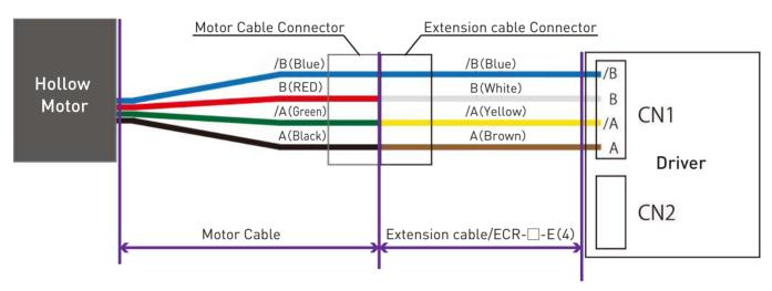
\*Please do not misplace each cable when using ECR-\(\subseteq=\text{E(4)}\) which they have different color from Motor cable, Please refer to the illustration above to connect each cable.
